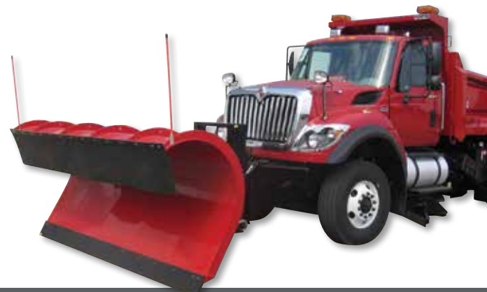
Slotted Trip Moldboard shown tripping over obstacle.
