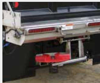
Self Leveling Spinner without Stabilizer Rod
