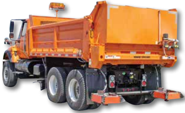
RTS Spreader with built-in Pre-wet Tank and Twin Spinner
