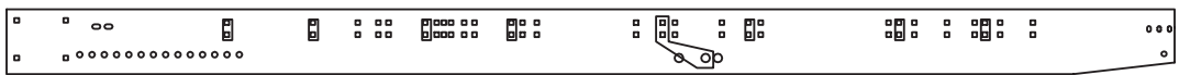
USE HOLES CONTAINED IN BOXES TO MOUNT CROSS BRACES FOR A 1000 GAL TANK SADDLE (00044179)
