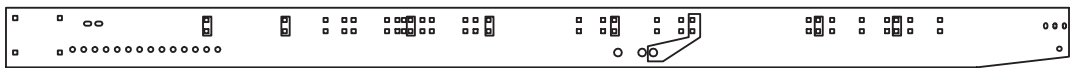
USE HOLES CONTAINED IN BOXES TO MOUNT CROSS BRACES FOR A 1235 GAL TANK (05050355)
