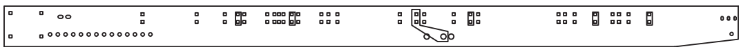
USE HOLES CONTAINED IN BOXES TO MOUNT CROSS BRACES FOR A 1300 GAL TANK (05052560)
