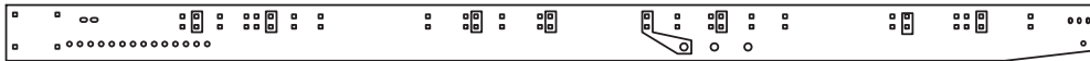
USE HOLES CONTAINED IN BOXES TO MOUNT CROSS BRACES FOR A 1600 GAL TANK (00048829)
