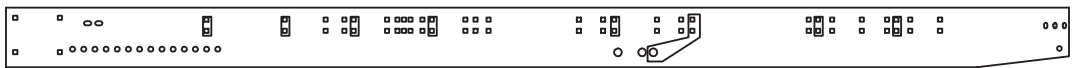
USE HOLES CONTAINED IN BOXES TO MOUNT CROSS BRACES FOR A 925 GAL TANK (05050721)
