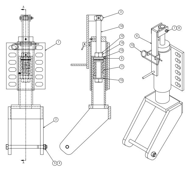
00106639 JACK ASSEMBLY, PLOW, SCREW, ROUND PNEUMATIC WHEEL
