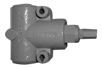
Down pressure relief is required on all Monroe underbody scrapers. A 500PSI relief can be incorporated into the truck hydraulic system or a down pressure relief valve can be purchased with the underbody scraper. The relief valve must be installed to prevent premature failure of the actuating cylinders and/or the underbody scraper.
