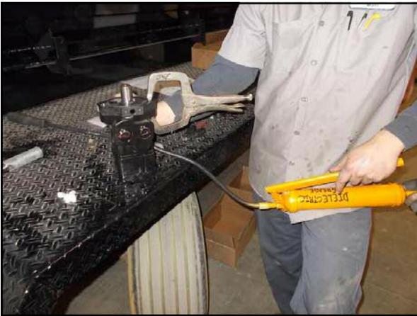
2. If installing grease before the motor and sensor are installed on the gearbox, lightly clamp the sensor block to the motor with a C-clamp. This will prevent the grease from pushing the block away from the motor.
