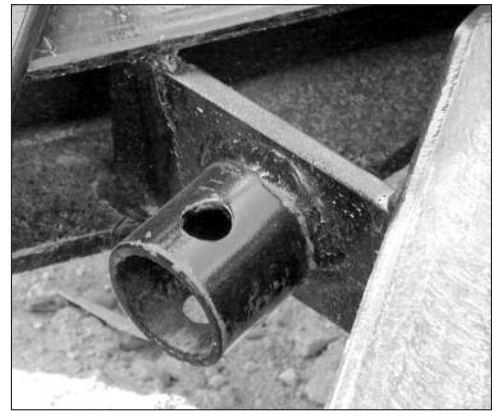
Tube and Bar are shown here mounted to the A-Frame
