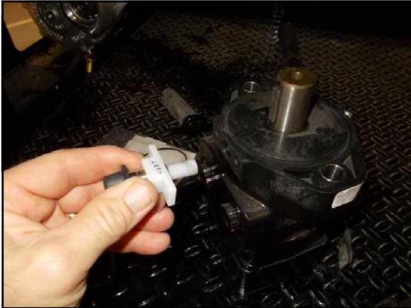
1. Remove the pickup from the sensor block.
