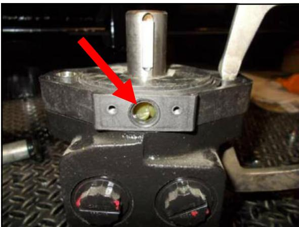
4. Pump grease into the block until it can be seen at the pickup opening. It is not necessary for the block cavity to be completely full of grease.
