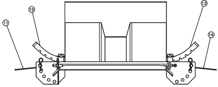
**00028001 CHUTE ASSEMBLY, SPINNER, LOWER, 20.0L X 20W**
