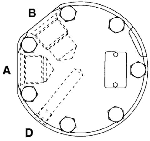
**PRESSURIZING PORT "B" RESULTS IN A CLOCKWISE SHAFT ROTATION AS VIEWED FROM THE SHAFT END.**
