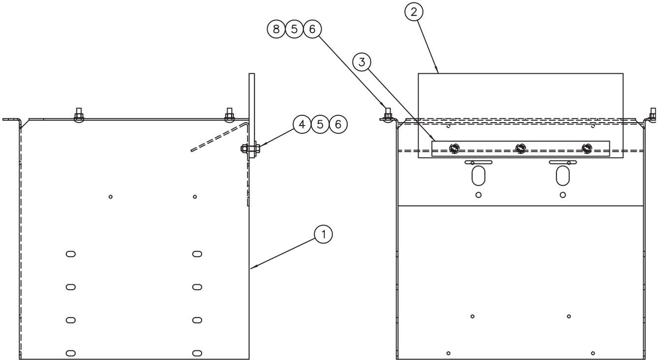
**00028044 CHUTE ASSEMBLY, BOLT-ON, V-BOX**
